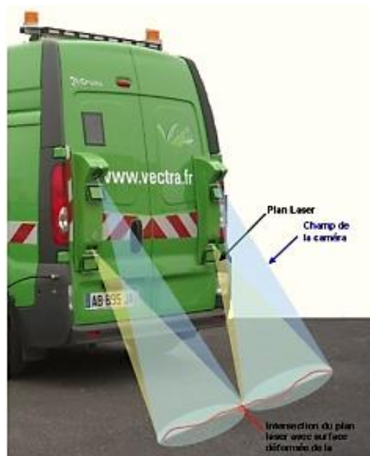
Principle of transverse profile sensors
