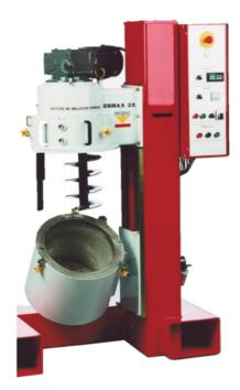
The BBMAX mixer, which complies with NF-EN 12697-35, allows preparing in laboratory relatively large samples of all coated materials for submission to subsequent tests on compaction, rut tester, circular shear press, module measurement, fatigue testing.
