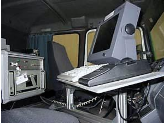
Cabin inside the Lacroix Deflectograph
