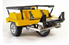
The GripTester measures a longitudinal friction coefficient (CFL) between the surface of the road and a tire with a braked wheel with a constant slip rate of about 15% close to the optimum of the anti-blocking system. This slip rate, which generates the adhesion force, is obtained by mechanical drive between the two carrier wheels and the measuring wheel.
