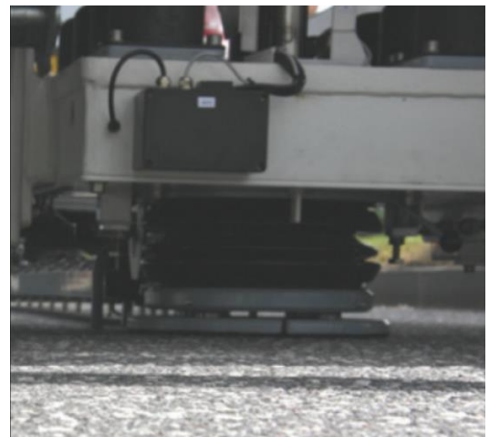
The four-split load plate allows full contact to the surface and accurate measuring.
